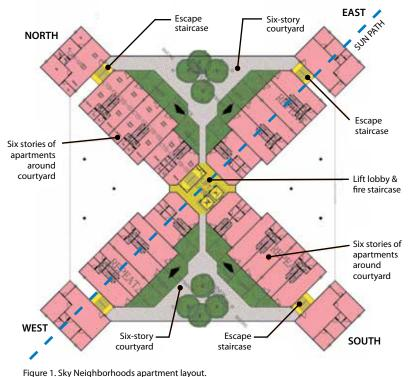
**66**The basic module in this layout comprises two doublestory apartments, which occupy three floors, one placed on top of the other, such that access to both apartment units is on the courtyard level, with the first unit connected to another floor below the courtyard level, and the second joined to another floor above the courtyard level.**99**
