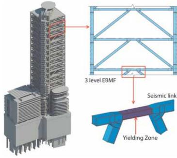
Figure 2. Overview of Eccentrically Braced Megaframe (EBMF).
