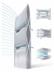
Figure 1. Sculpted façade directing wind through the vertical axis wind turbine (VAWT)
