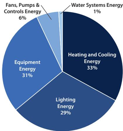
▲ Figure 1: Average energy consumption of a typical high-rise office building. (Source: Interpreted from the US Department of Energy's reference building energy models for existing large commercial buildings built after 1980, across 16 US cities, in various climates.)
