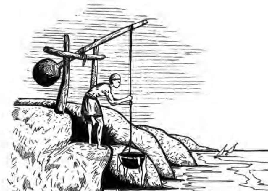
Figure 1.1.1. A representation of the Egyptian Shadoof , which used a cantilever system to collect water or lift heavy objects, circa 20th century BCE. Source: Travelers in the Middle East Archive , redrawn by Gianluca Contran
