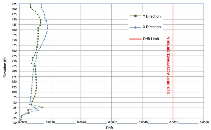
▲ Figure 6.3: Max SLE Seismic (Site-Specific) Story Drift. © Magnusson Klemencic Associates
