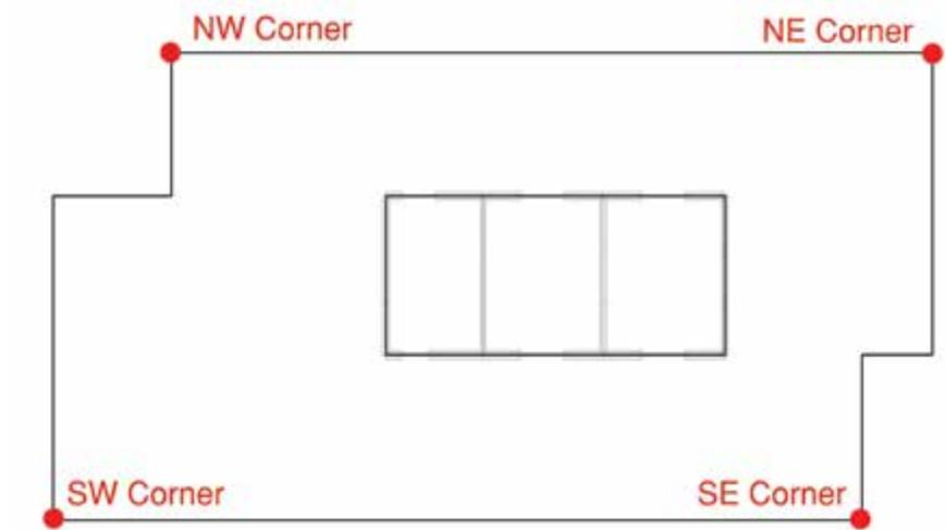
▲ Figure 6.2: Example Corner Points for Drift Determination. © Magnusson Klemencic Associates
