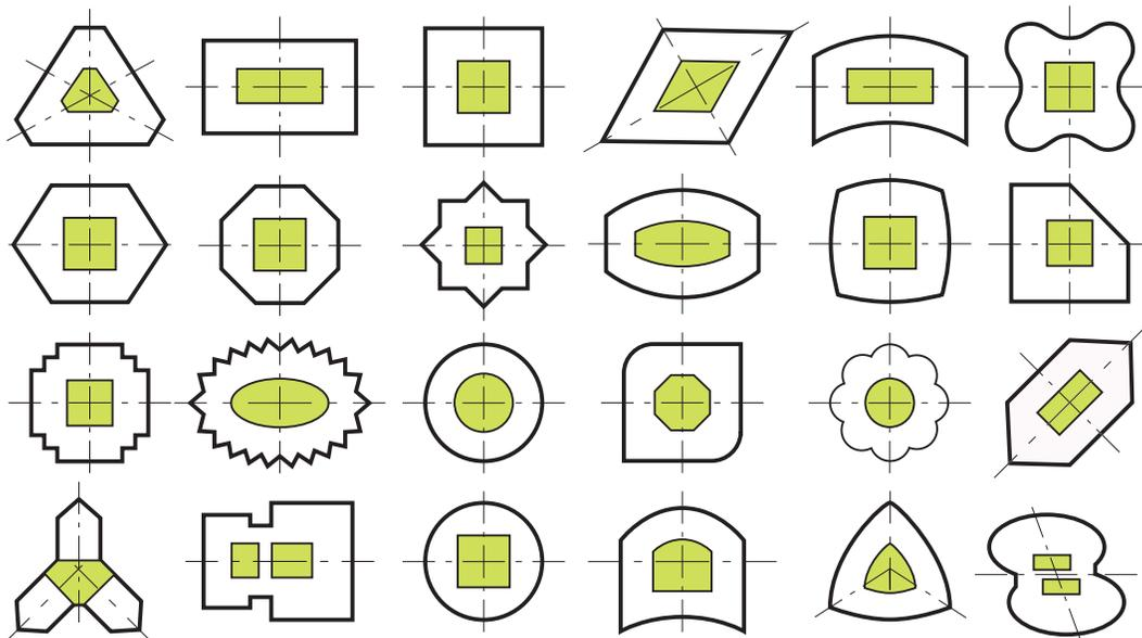
Figure 1.1. Various building shapes used in supertall buildings, with the core location identified in green. © WSP, redrawn by CTBUH
