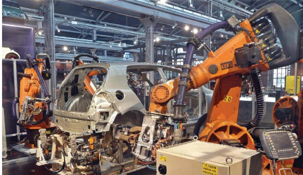
Figure 4.3.1. Some industrial robots, like these automotive assembly arms, are designed to work fully separated from human workers for safety reasons. © Norbert Kaiser (cc by-sa)
