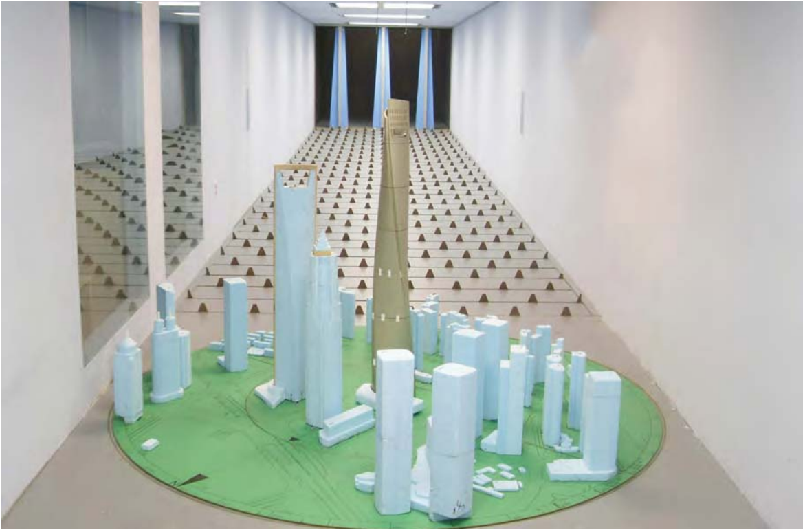
▲ Figure 3.1: Shanghai Tower, Shanghai, China. Wind tunnel test performed in March 2009. © RWDI
